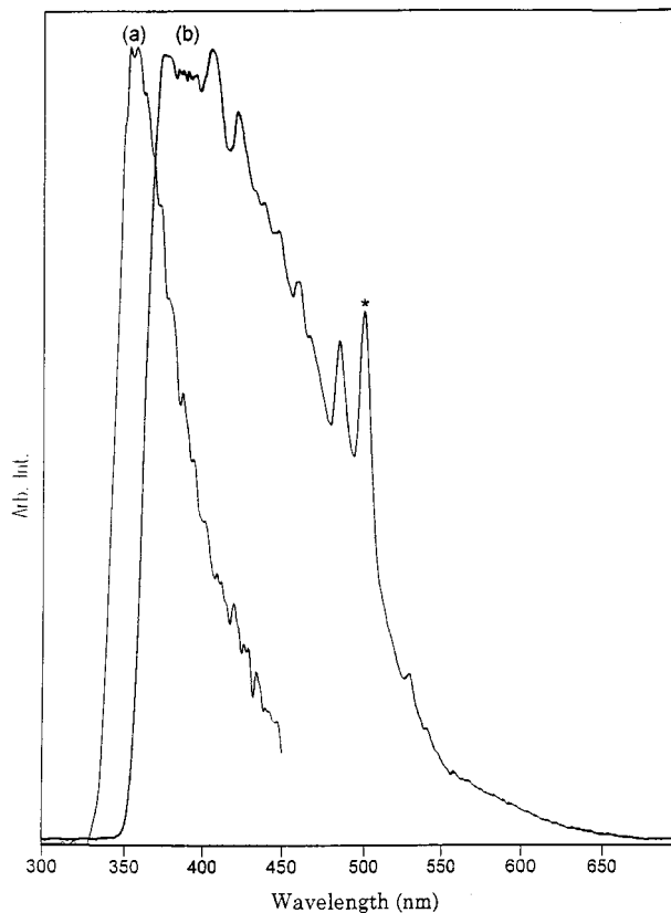
Fig. 2. The changes of emission spectrum of cis -stilbene in the sol-gel system: (a) initial liquid, (b) dried gel. The peak labeled with the asterisk is due to the second-order signal of the excitation line.
